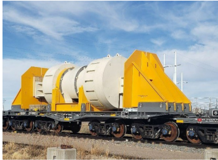
Figure 7. Atlas railcar loaded to a maximum 240-ton (480,000 pound) test load designed to simulate the heaviest transport container certified by the NRC. Modified from (Bickford 2023)
