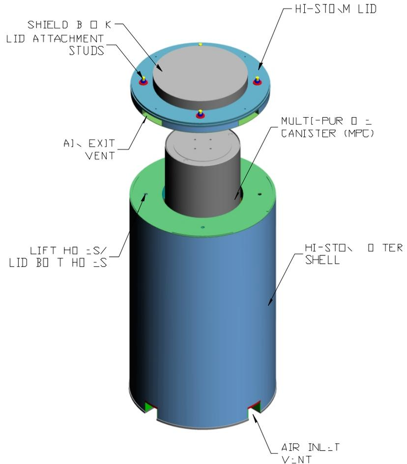
being used, the water also is drained from the canister. The lid then is bolted or welded in place, and operations to dry the fuel are started.
