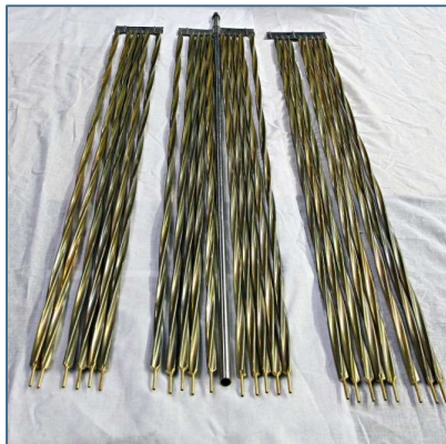
Mockup of 4-lobe helical cruciform fuel rods.
