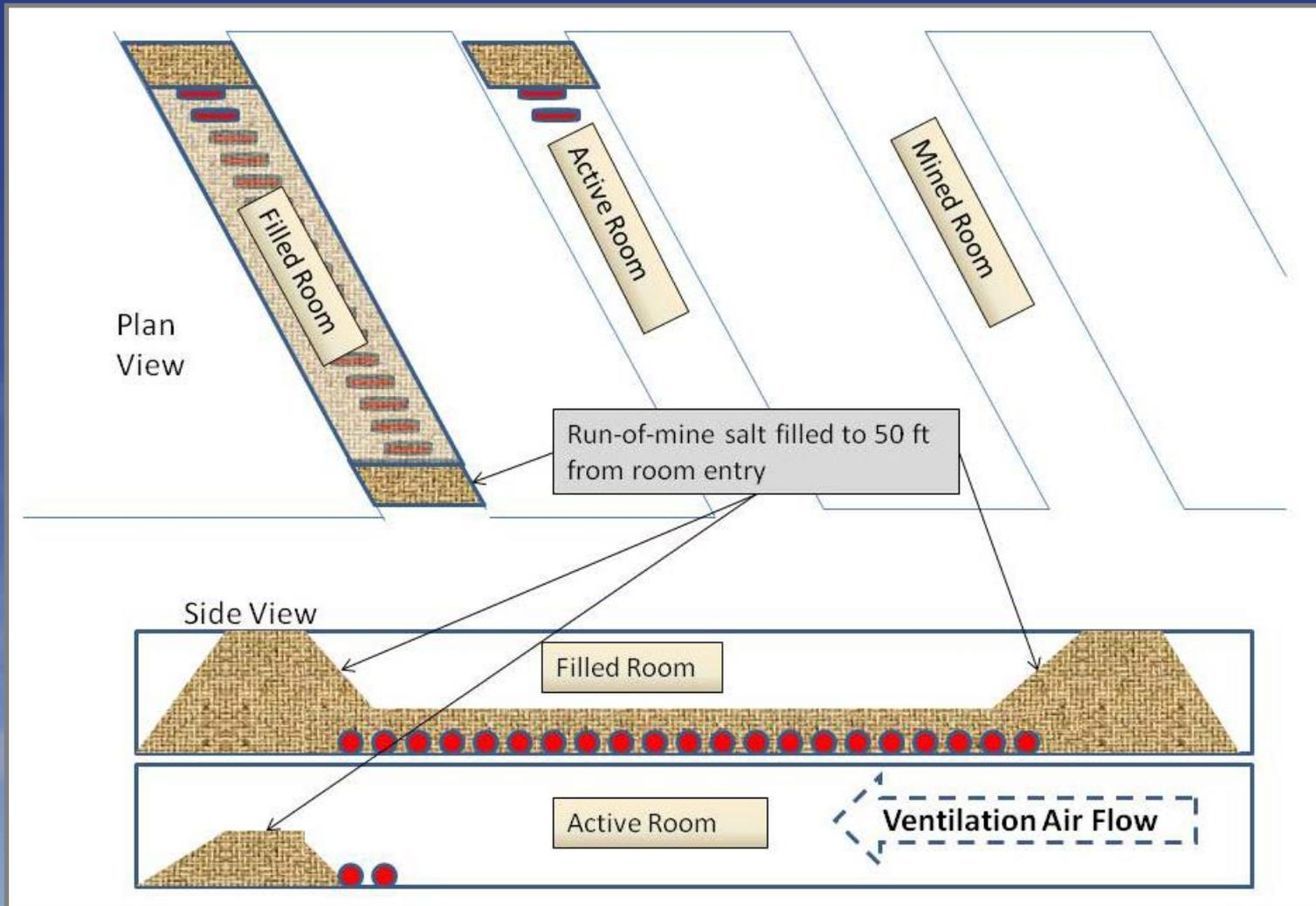
Emplacement concept adapted from Carter, J.T., et al. (2012). "Reduced Backfilling and Backfilling." *Defense Waste Salt Repository Study*. DOE Office of Nuclear Energy Report ORNL/D-2012-000116.
