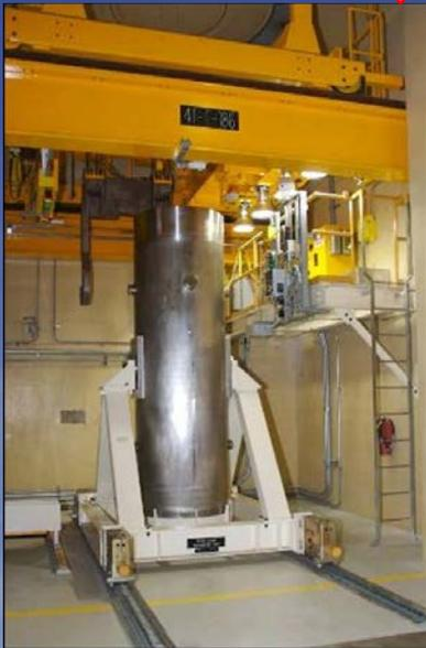
Waste canisters pulled from shipping cask behind shield doors and placed into shielded facility cask for handling
