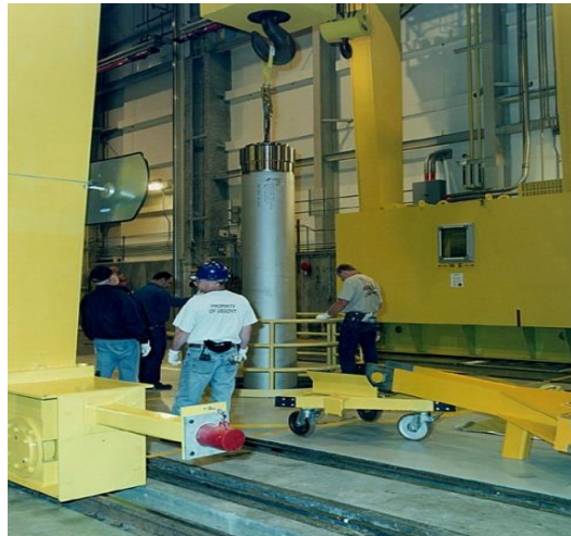
Left: CSB interior. Center: Empty MCO loading into cask at CSB. Far Right: CSB vault construction.
