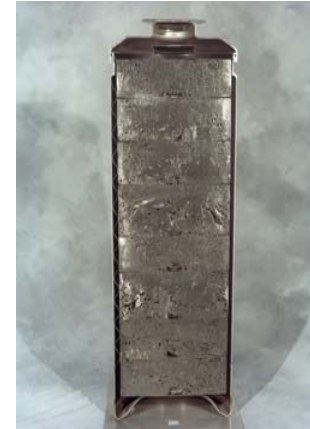
Compacted Hulls and End Pieces
