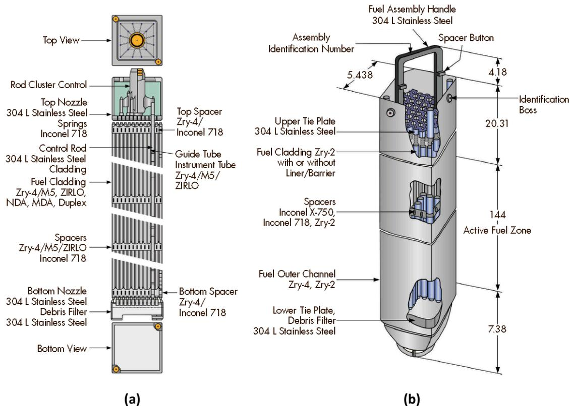
**Figure 5. Examples of (a) Pressurized Water Reactor and (b) Boiling Water Reactor Fuel Assemblies (Strasser et al. 2014).** Provided by Courtesy of ANT International. Dimensions in Inches.
