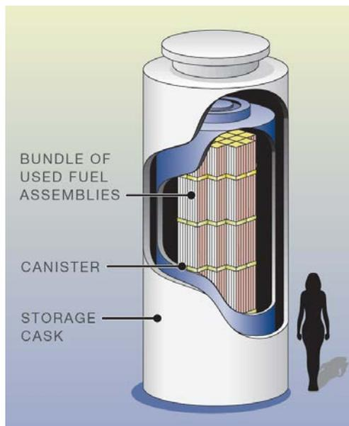
**Figure 2. Spent Nuclear Fuel in a Dry Cask Storage System.** Source: BRC (2012).
