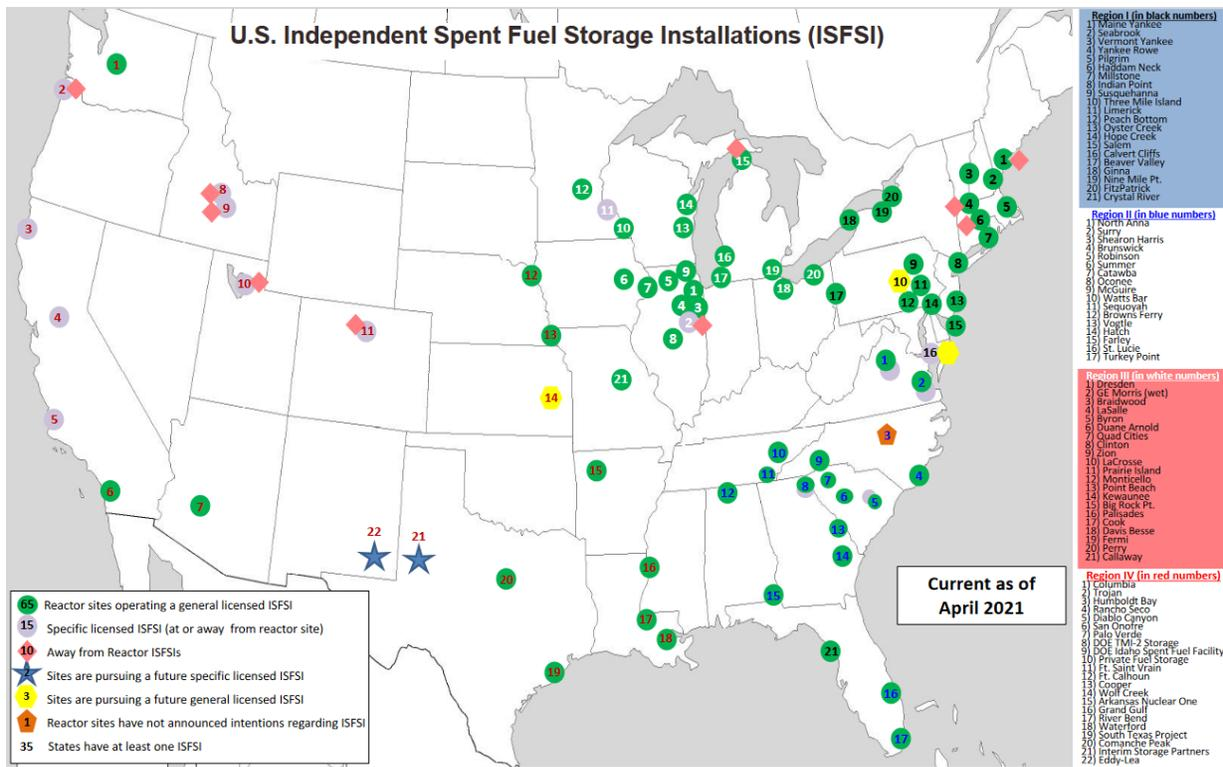
Figure 4. Locations of U.S. Independent Spent Fuel Storage Installations. Source: NRC (2021d).
