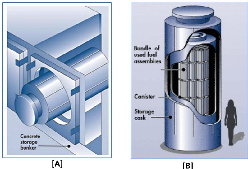
**Figure 1. Dry Cask Storage Systems for Commercial SNF.**
