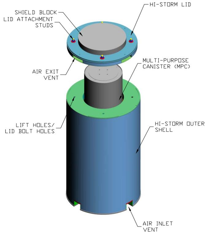
**Figure 4. Typical Vertical Dry Cask-Storage System**
