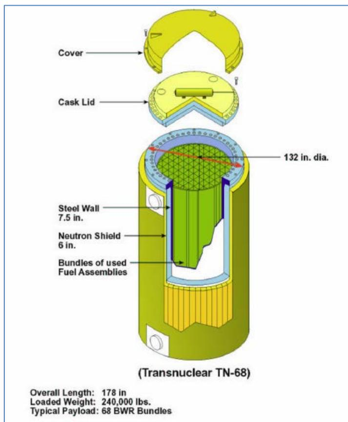
Figure 1. Typical Dry-Storage Cask (NRC 2011)
