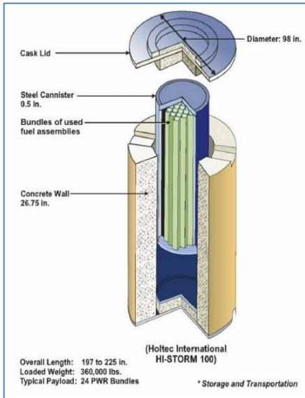
*Figure 2. Vertical Concrete Overpack (NRC 2011)*
