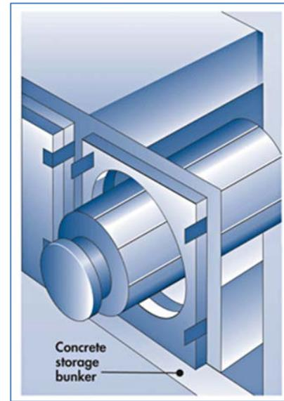
*Figure 4. Horizontal Concrete Bunker (NRC 2013)*
