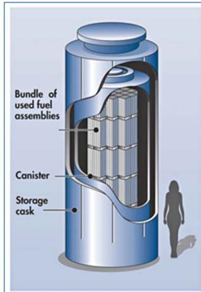
*Figure 3. Vertical Metal Overpack (NRC 2013)*
